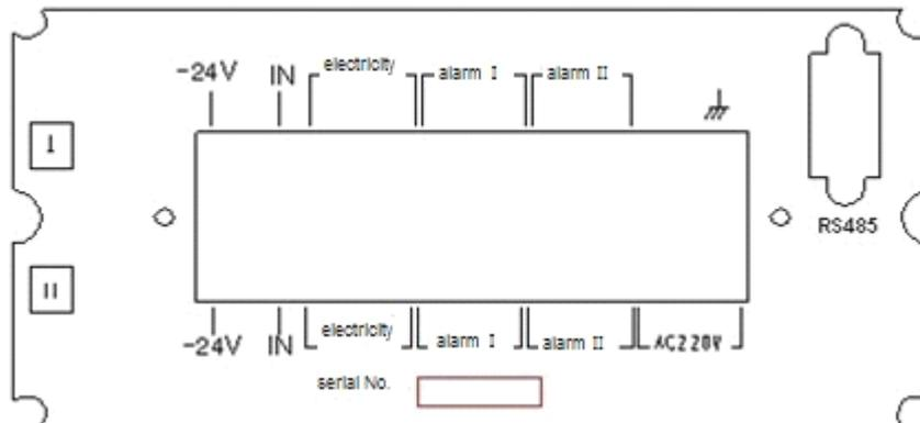
**Figure: Wiring Diagram for YD420 Intelligent Shaft Vibration Monitor**
