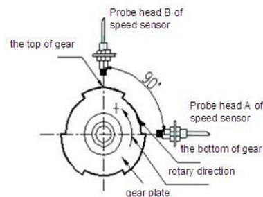
The drawing of sensor installation
