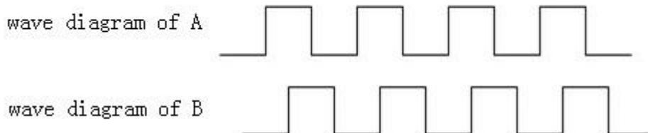
As shown above Sensor A wave line surpass Sensor B wave line 90 degrees.
