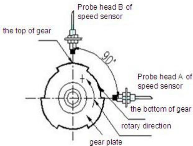
As shown above when the mechanical rotate to the counter-clockwise direction (assumed to be forward) , the sensor waveform is as following:
